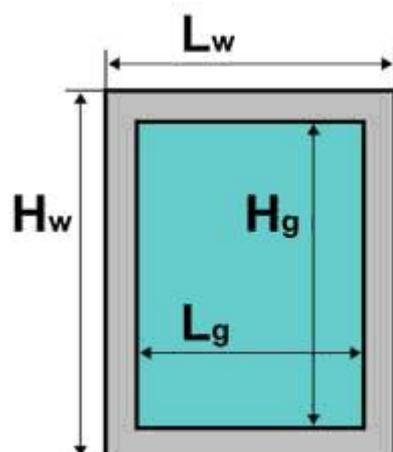
$$\begin{aligned} L_w &= 0,50 \text{ m} \\ H_w &= 1,10 \text{ m} \\ L_g &= 0,40 \text{ m} \\ H_g &= 0,90 \text{ m} \end{aligned}$$
