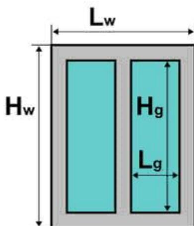
$$\begin{aligned} L_w &= 1,36 \text{ m} \\ H_w &= 3,60 \text{ m} \\ L_g &= 0,55 \text{ m} \\ H_g &= 3,40 \text{ m} \end{aligned}$$
