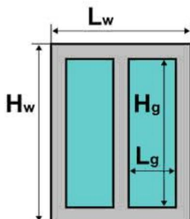
$$\begin{aligned} L_w &= 1,10 \text{ m} \\ H_w &= 1,60 \text{ m} \\ L_g &= 0,45 \text{ m} \\ H_g &= 1,40 \text{ m} \end{aligned}$$
