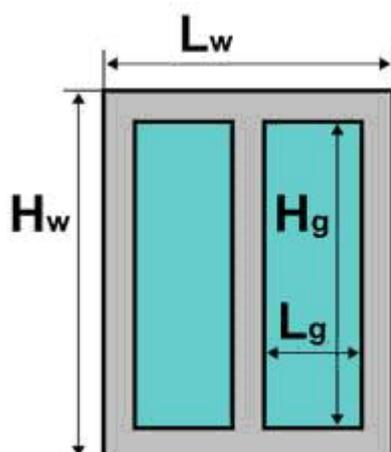
$$\begin{aligned} L_w &= 1,20 \text{ m} \\ H_w &= 2,50 \text{ m} \\ L_g &= 0,50 \text{ m} \\ H_g &= 2,30 \text{ m} \end{aligned}$$
